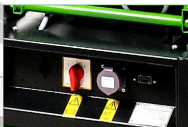
Extra operating panel integrated in chassis with battery indicator
